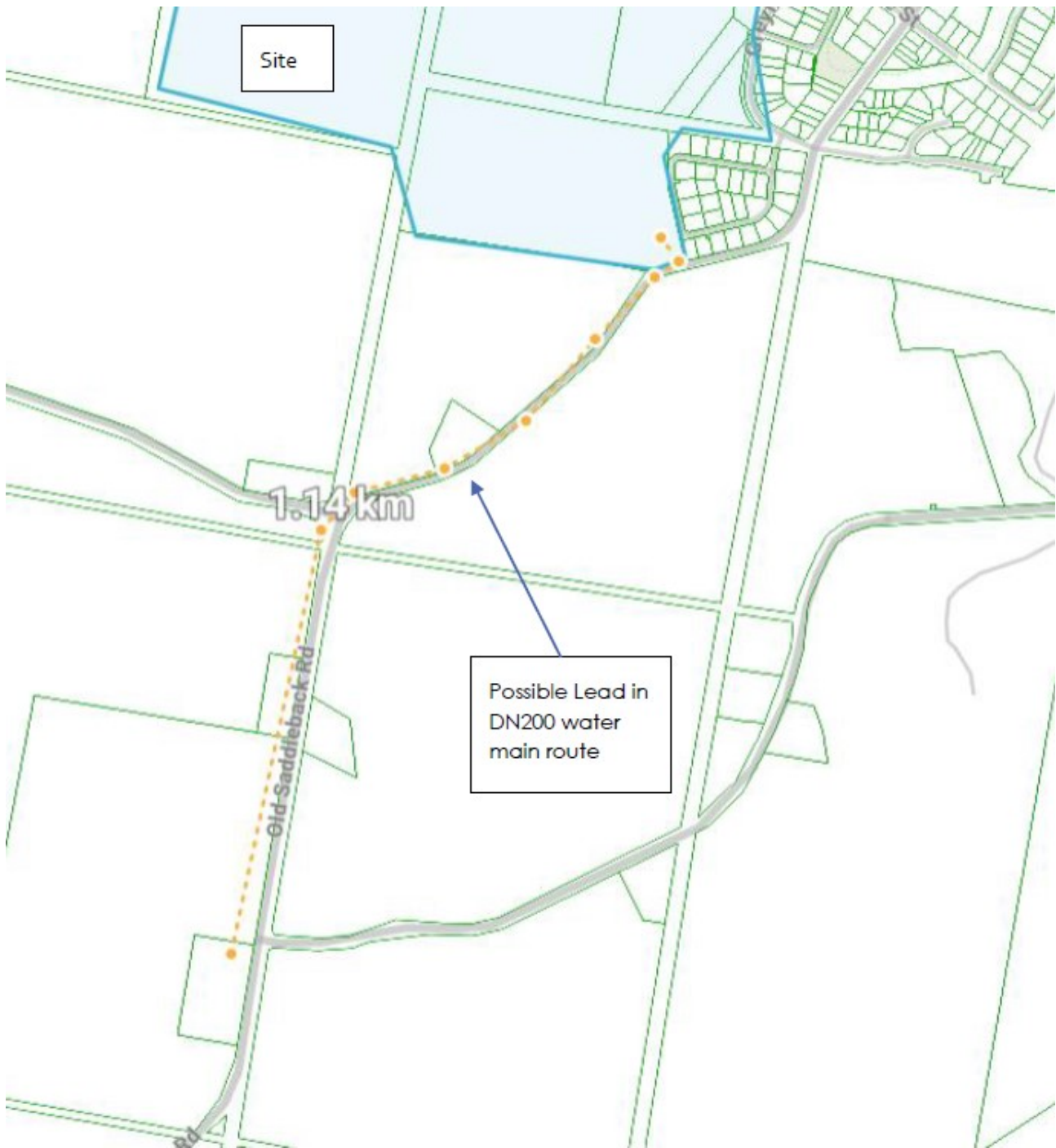
Figure 7 – Lead in potable water main to service land above RL 82
