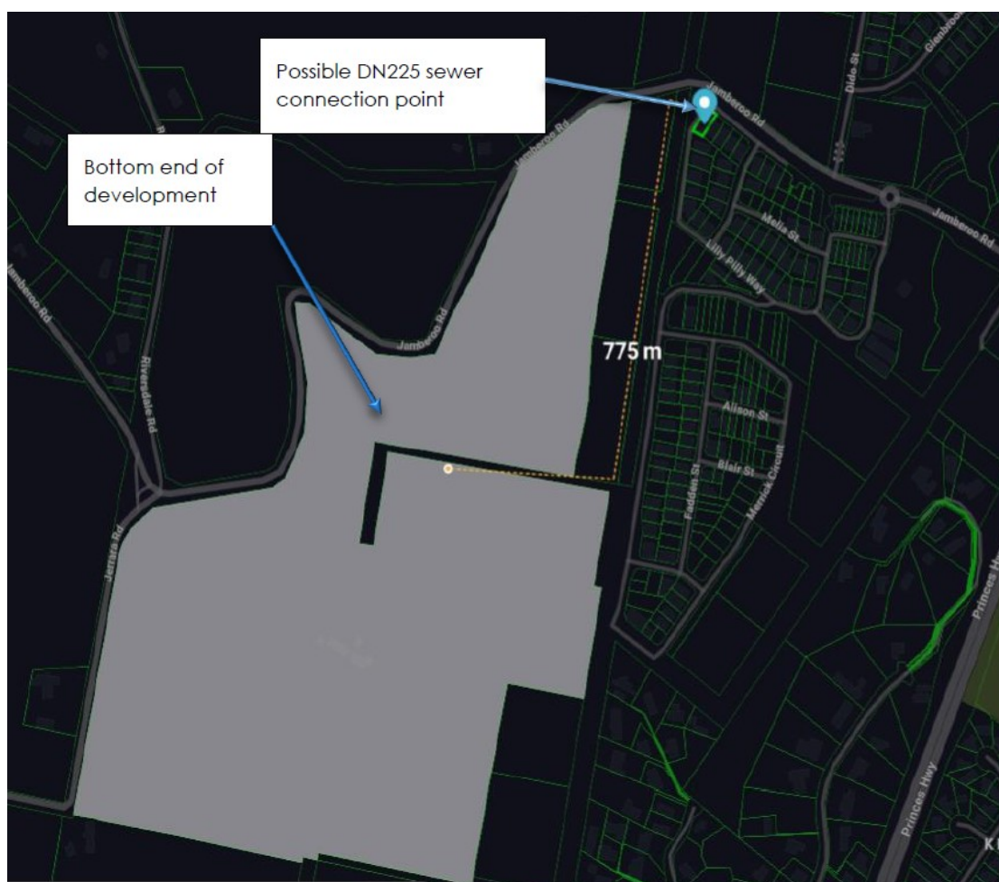
Figure 8 – Location of nearest downstream DN225 sewer
